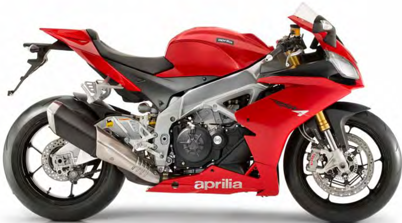
Forged aluminum front wheel rims
